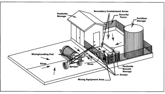
**Figure PHF-1.** Example Combined Pesticide and Fertilizer Storage and Mixing Area. Figure courtesy of *Designing Facilities for Pesticides and Fertilizer Containment*, Midwest Planning Service, Agricultural Engineering, Iowa State University 1991.
